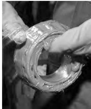
Fig. 15. Grease can easily be packed by hand.
