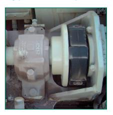
The CENTAFLEX couplings have been proven in many areas of mechanical engineering. The major area of application lies with diesel driven stationary and mobile
