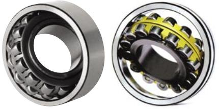
Spherical Roller Bearings have two Raceways on Inner Ring, and one Spherical Raceway on the Outer Ring. As the name implies, the Rolling Elements of the Bearing have a spherical profile.
