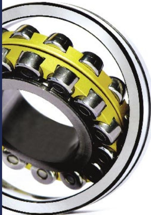
The material for KG Rolling Bearings is normally high Carbon, thorough-hardened Chromium Steel with a good degree of cleanliness. For special applications that involve shock loads and reverse bending stresses, certain Bearings made with case-hardened Steel are also available.
