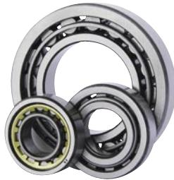
As the name implies, these Bearings have Cylindrical Rollers as Rolling Elements. They form a line contact with the Raceway of Inner and Outer Ring. KG Cylindrical Roller Bearings are produced in many variants, and can also be made as per special dimensional requirements, but within some basic design limitations.
