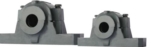
Plummer Block Housings help to form Bearing units, with Self-aligning Ball Bearings & Spherical Roller Bearings. They permit flexibility in the choice of Bearing, location on Shaft, Seals & lubrication. Made on modular principle using Cast Iron HT 200 JIS 5501, KG Housings are available in a wide range of sizes to suit various application requirements.
