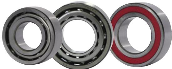
Angular Contact Ball Bearings are similar to Deep Groove Ball Bearings, however they can sustain combined radial & axial loads, because the line of contact between the Balls & Raceway is at an angle in the radial plane.
