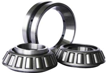
The Rolling Elements of this Bearing are Tapered Rollers. They form a line contact with the Raceway of Inner Ring and Outer Ring (Cup). These are separable type Bearings. Tapered Roller Bearings can also be made according to special dimensional requirement, but within basic design limitations. They are available in both metric and inch dimensions.
