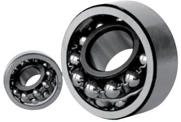
The Inner Ring of Self-aligning Bearings has two Raceways, and Outer Ring has one spherical Raceway with its center at the axis of Bearing. These Bearings have a self-aligning character, hence the name.
