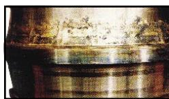
the lubricant. Friction due to rotation slow down leads to a temperature rise and consequential expansion leads to Seizure between the Rolling Elements and Raceways.
