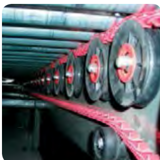
PowerMax V-Belt Idlers used with PowerTwist Roller Drive on a Live Roller Conveyor.
