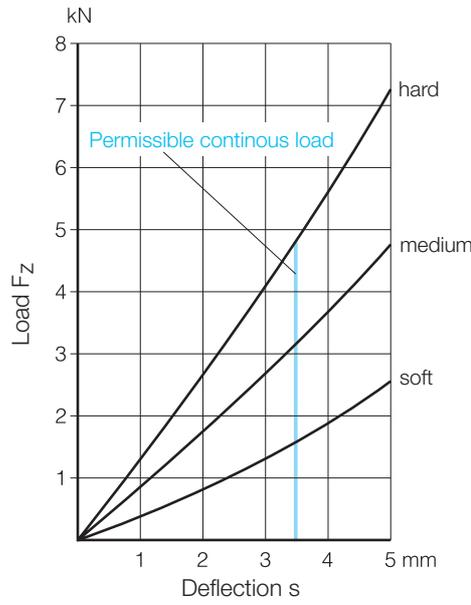
**Megi Machine Mounts with height adjustment**
