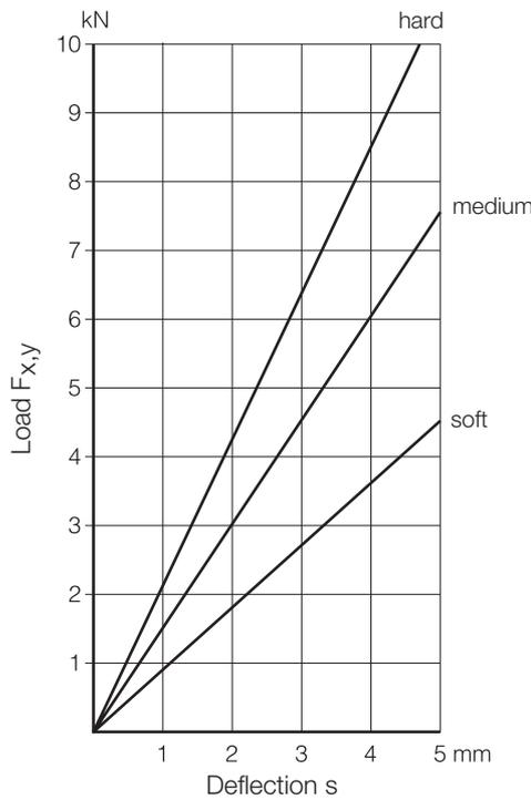
**Megi Machine Mounts with tear-off protection**
