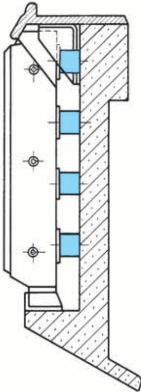
Megi stop bumper with intermediate plate vulcanised end, fitted into fender element on pier.
