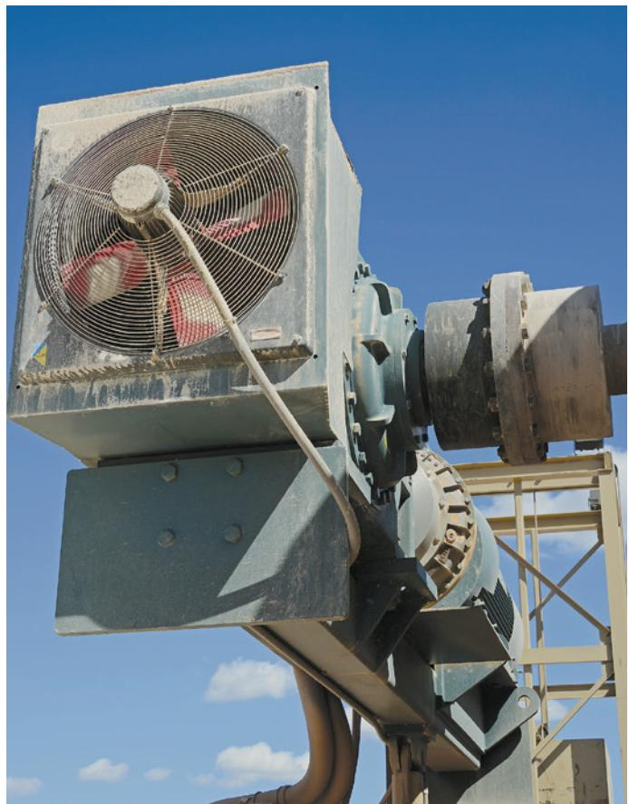
The Dodge DM Moment coupling is specifically designed to make the rigid connection between the output shaft of the gearbox and driven equipment.
