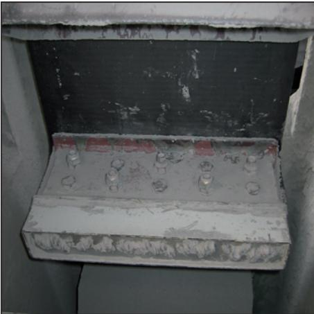
Metal clamps are the most common method for elevator joining. Typical application is shown on the left. Vulcanized splicing are possible too; the efficiency is very high but the vulcanization in vertical position needs special procedures, tools and skilled people.
